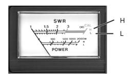
Thank you for purchasing your Power/SWR Meter from *RadioShack*. Measuring SWR shows you how much of your radio's transmit power is reflected from the antenna back into the antenna cable and lost. With this information, you can adjust the length of your antenna or antenna cable so your antenna and radio combination can operate at maximum power. Please read this user's guide before installing, setting up and using your new meter.
