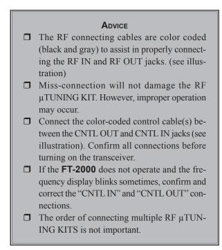
The RF uTUNING KIT provides ultra-sharp RF selectivity for the front end of the transceiver. Very high O is made possible by the narrow-band design. Three RF µTUNING KITS are available. The MTU-160 covers the 1.8 MHz band. The MTU-80/40 covers the 3.5 and 7 MHz bands. The MTU-30/20 covers 10.1 and 14 MHz bands.
